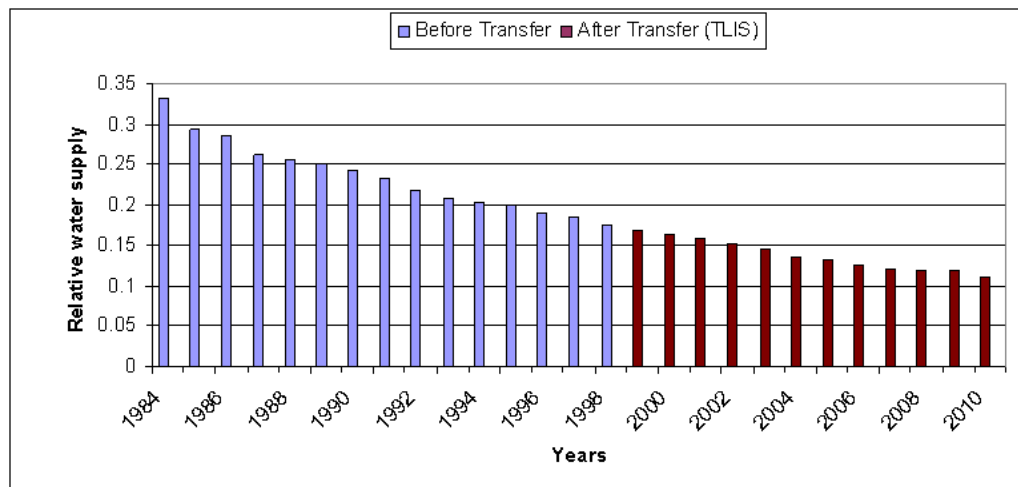
Fig. 8 Relative water supply of the Takari Lift Irrigation Scheme for the pre- and post-transfer periods
