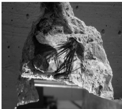
Fig. 6 Brittle failure of the CFRP pretensioned rebar in the concrete slab
