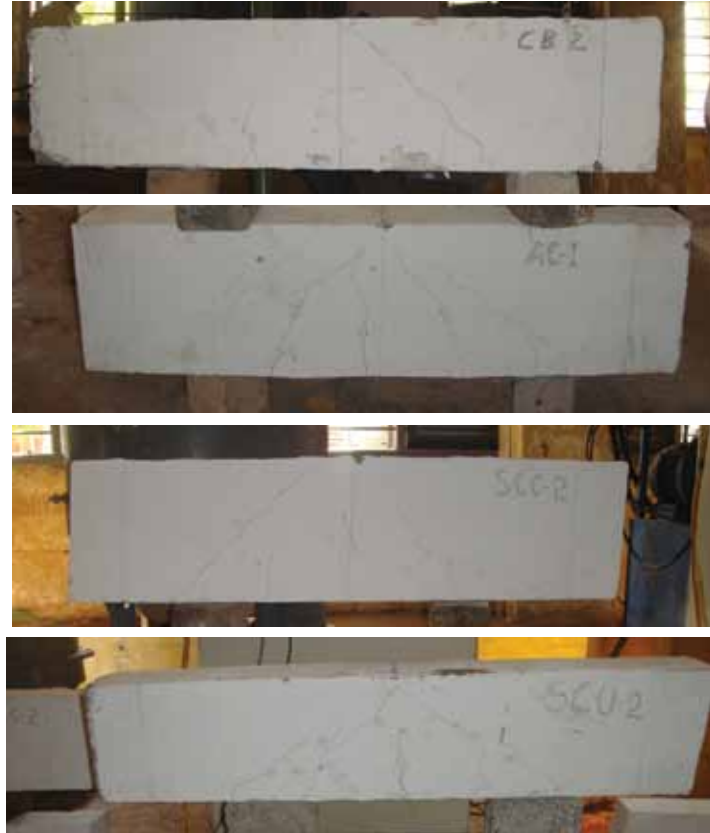
Fig. 7 Failure of All Specimens
