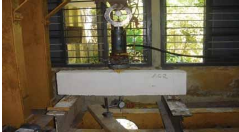
Fig. 5 Static load set up for beams
