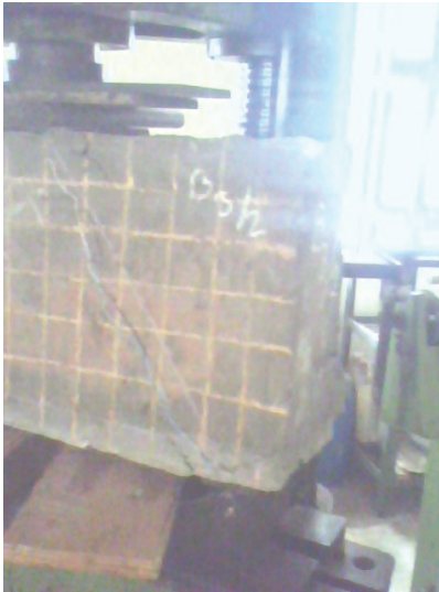
Fig. 7 Deep beam testing
