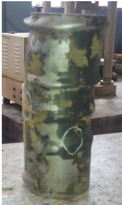
Fig. 6 Failure of normal mortar Steel tube
