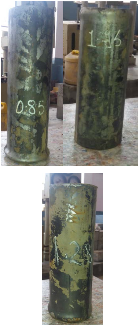
Fig 7 Failure of Aerated mortar
