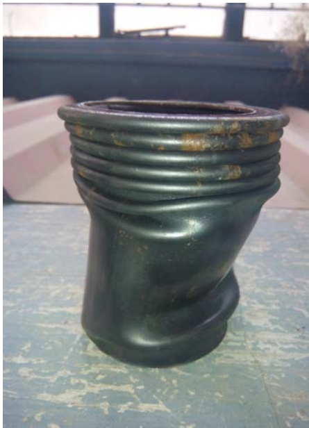
Fig.5 Hollow steel tube after failure on U.T.M.
