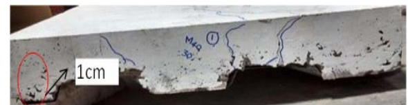
Fig. 15 Slip behaviour for slab 30°
