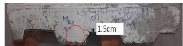
Fig. 14 Slip behaviour for slab 15°
