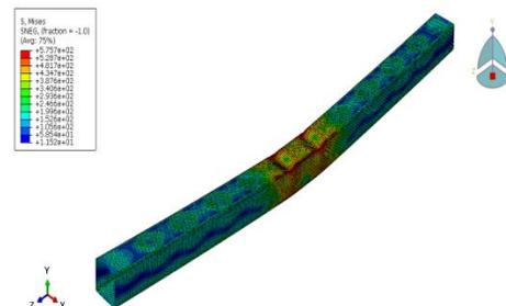
Fig. 4 Deformation shape for the section 50x50x1.0xM1
