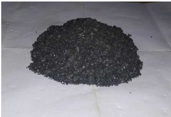
Fig. 2 Appearance of Copper Slag used for the Stabilization
