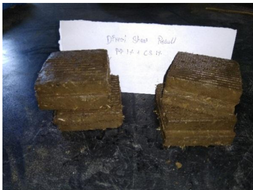
Fig. 5 Failed Sample Obtained from the Direct Shear Test
