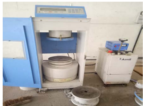
Fig.5 Compression Testing Machine (CTM)
