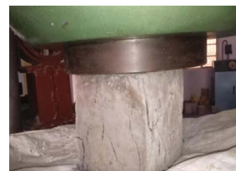
Fig. 2 Failure pattern of Cub
