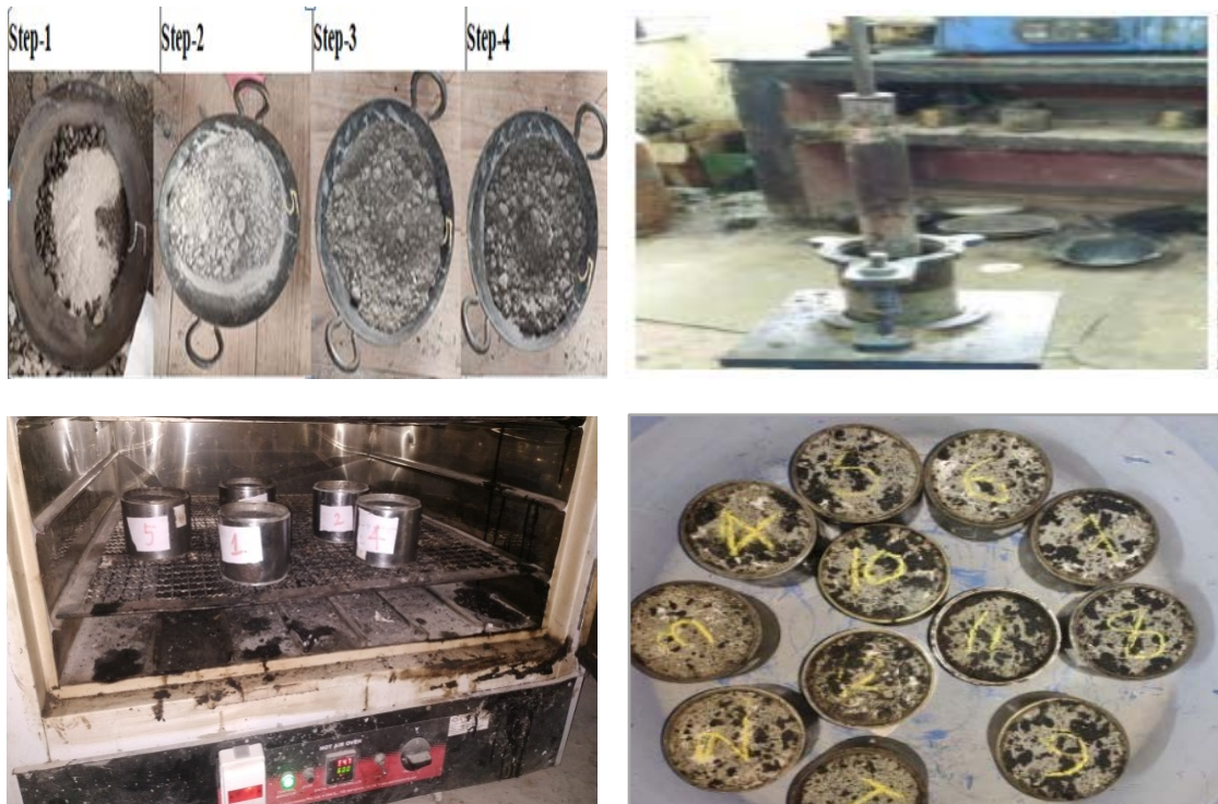
Fig. 2 Cold Mix Design (Sample preparation)
