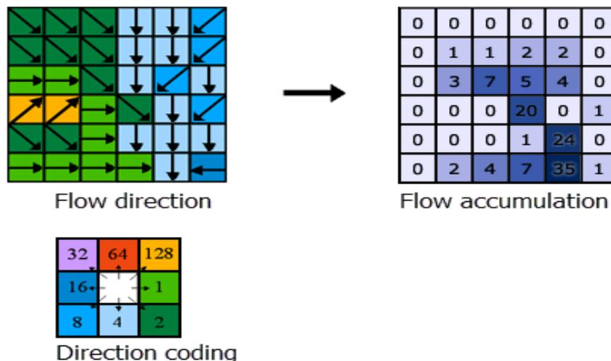
Fig. 6 Determining the accumulation of flow
