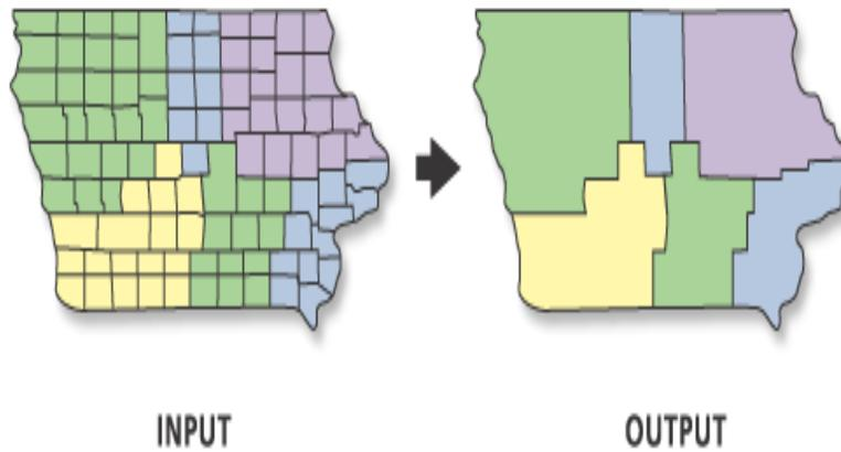
Fig. 14 Principle of Dissolve Tool
