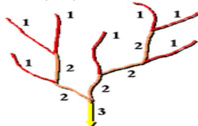
Fig. 10 Strahler stream ordering method
