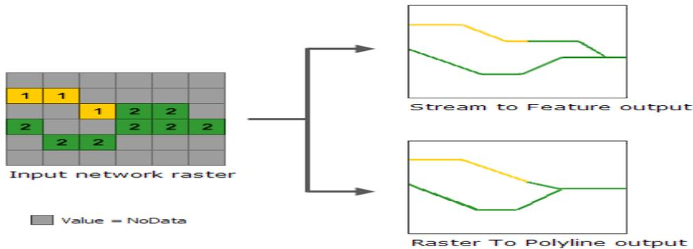
Fig. 12 Comparing vectorizing stream network raster methods
