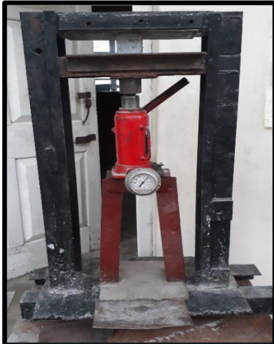
Fig. 2 Arrangement for compressive strength analysis
