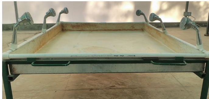
Fig. 2 The heap leaching setup used in the heap leaching study
