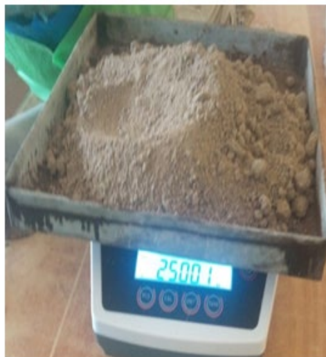
Fig. 5 Initial weighing of fine aggregate
