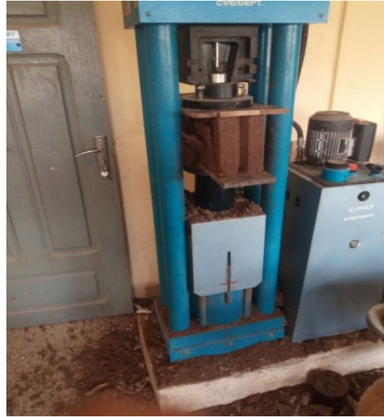
Fig. 7 Sandcrete blocks ready for crushing
