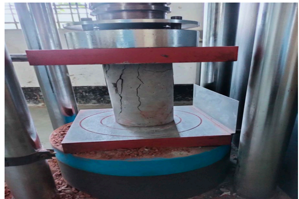
Fig. 6 Compressive strength test
