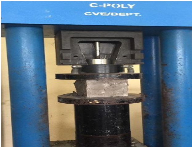
Fig. 10 Specimen under compressive strength test
