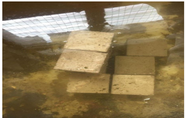
Fig. 8 Curing of specimen
