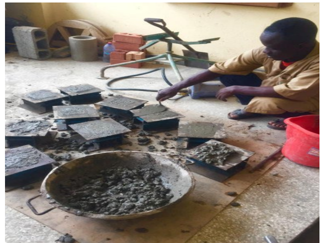
Fig. 7 Casting of specimen
