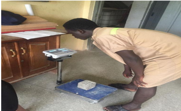
Fig. 9 Weighing of specimen
