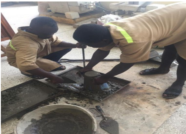
Fig. 6 Conducting a slump test
